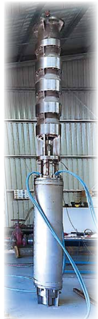
1 of 4 x 14" 330kW Super Duplex SS motor and pump
